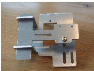
Do **NOT** fit the motor before doing this as you will not be able to get the slider in once the motor drive pin has been fitted.
