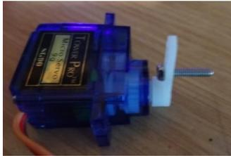
Screw the M2x6mm screw through this hole from the back (motor side). If the hole is a little too big, add a M2 nut to the front to make it secure.
