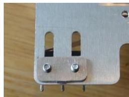
Fit the switch to the slots with 2 x M2x10mm screws and the tapped nut plate.
