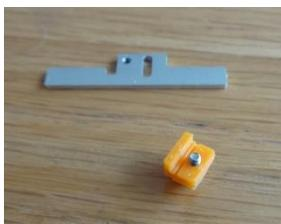
Make up the slider by fitting the wire clip (orange plastic part) with the M2 x 4mm screw in such a way that the raised edge fits along the side in the groove provided. (for point motor)
