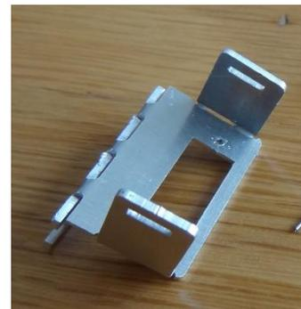
The 2 wings are bent in the opposite direction and can be bent by hand on a wooden block.
