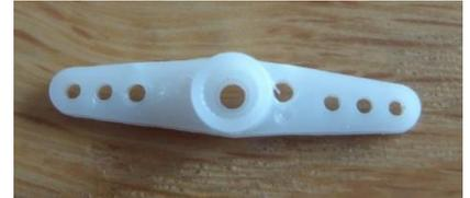
Note: you can cut off the other side of the horn if required as this is not needed for the final mount.
