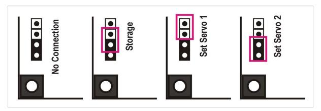
With setting Jumper moved to top position you can set Servo 1 (White Setting Pins) Immediately the White LED will flash twice and then go out indicating that the board is now in setting mode.
