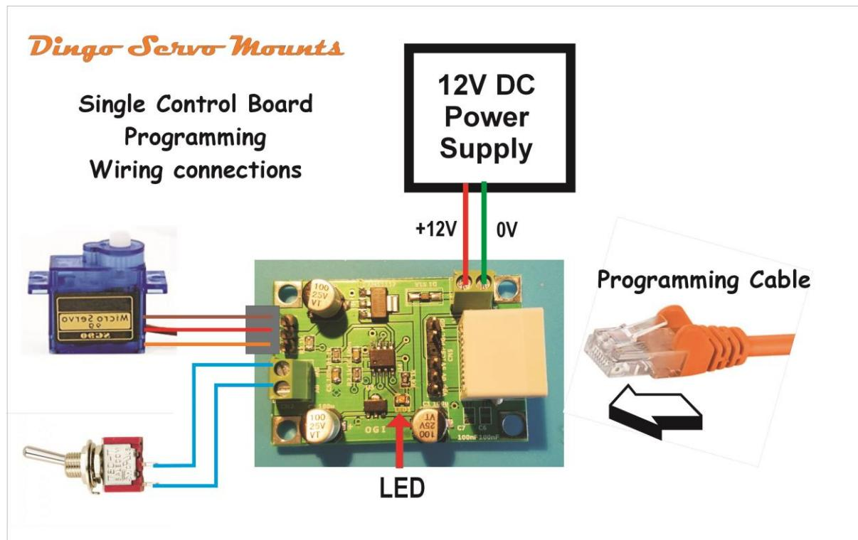
Now plug one of our setting boxes into the RJ45 connector on the board.
