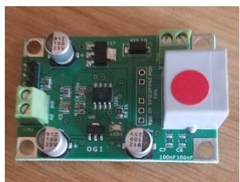
**Note: A RED dot on the PCB indicates that the firmware has been updated to be compatible with the Ultra Micro Servos: HK5330 and HK282A as well as operating normal 9g servos. (HK15178, SG90, etc)**
