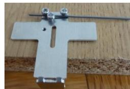
The unit is designed to accommodate up to 4 microswitches fitted with M2 screws and nut plates into the 4 slots at the “bottom” of the unit. 2 switches are included in the kit, but more can be ordered separately.
