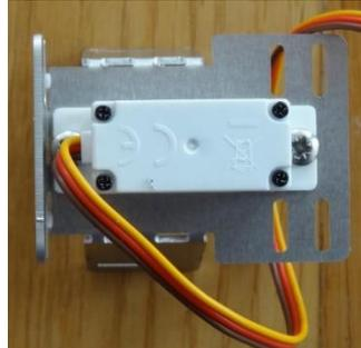
Now the servo motor needs to be centred by means of a servo tester or the control software.
