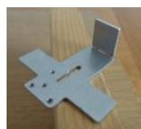
This fold is required for operating the switches if fitted. (If you fold this one the wrong way, it will just mean that your actuator wire will be on the other side of the mount, but will still function fine.)
