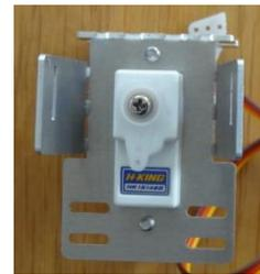
Attach with the small screw provided by the servo manufacturer so that the long part points down
