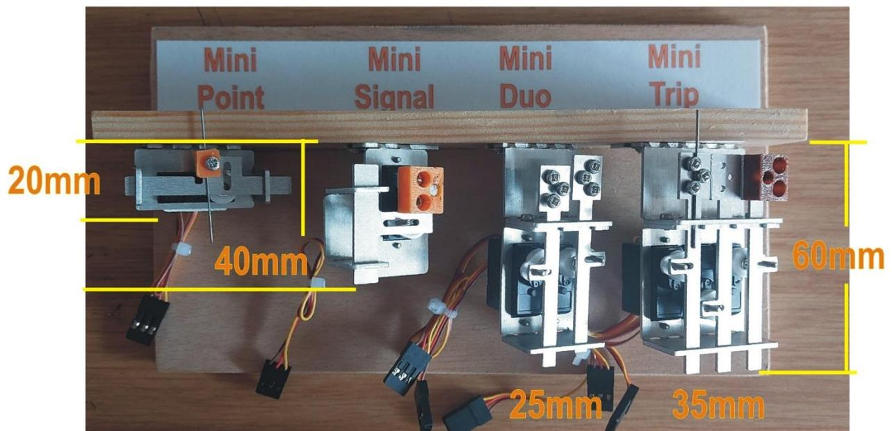
**A Mini Point.** This features a small point mount styled on the Ultra Micro idea. (N gauge or smaller)
