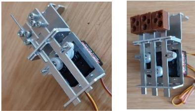
Because the actuator horns supplied with these smaller servos are a bit fragile, I include a 3D printed horn (Boss) to use instead. This horn is designed to hold the M1.6 x 8mm screw which acts as the drive for the servo to the slider.
