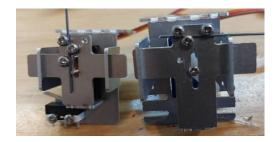
This is the first prototype which will accommodate the Power HD HD1370A servos which we use in all the mini mounts.
