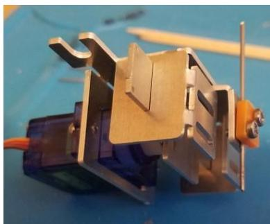
At the moment this mount will be less than 25mm under the baseboard and will be able to operate 2 switches. I am hoping to get this down to less than 20mm if possible and also make is able to operate either as a point motor or a signal driver much like the Ultra Micro Mount.
