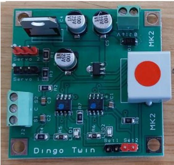
I have had a couple of issues with the twin servo board, usually when the servos have been overdriven against an obstruction which has caused the main regulator to fail. This board has now been redesigned with a larger regulator on board to alleviate this.
