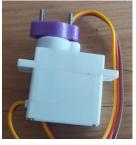
Next centre the servo with a servo tester or other means and then fit the drive boss onto the servo shaft making sure that it is square and not catching anywhere.
